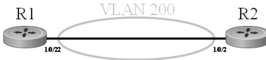
Figure 238 Diagram of a Routed VLAN
