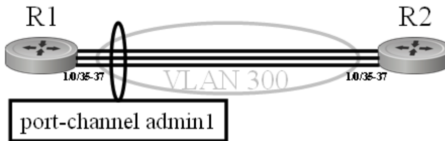
Figure 170 Adding a LAG to a VLAN
